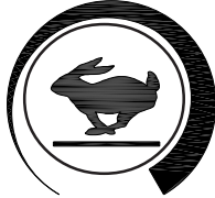
Traverse Speed Control ("L Class")
